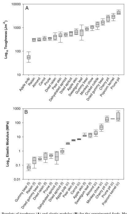
Fig. 3. Boxplots of toughness  $(\mathbf{A})$  and elastic modulus  $(\mathbf{B})$  for the experimental foods. Means are indicated by the line. The 5th and 95th percentiles are indicated by the whiskers. The data are logged to facilitate the graphical representation.
