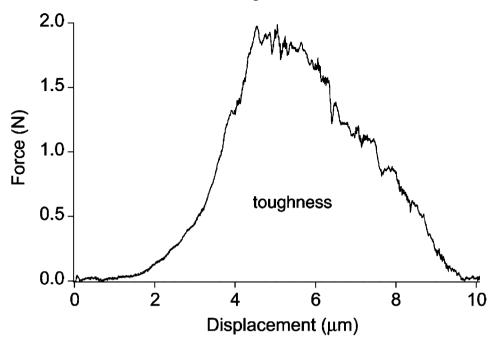
Fig. 2. Force-displacement graph for a raisin sample measured using the scissors test on a portable mechanical-properties tester. Toughness is equivalent to the area under the force-deformation curve divided by the area of new crack growth. It is an indication of the amount of work per unit area (Joules per square meter) done on the material during fracture.
